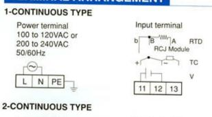
Power terminal 100 to 120VAC or 200 to 240VAC 50/60Hz
